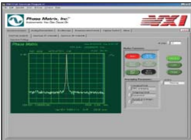
Figure 3. 5 GHz CW signal observed via a spectrum analyzer synthetic instrument.
